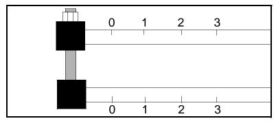
Figure 3-8: Fixture with Scale Origins Properly Aligned
